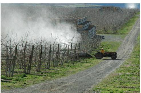
Picture of orchard air blast sprayer applying an early season spray
